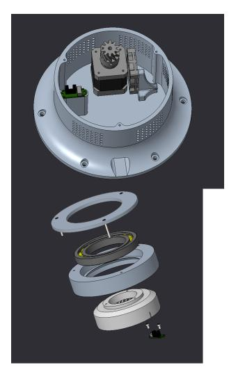
Firstly the motor is screwed to the basebot. Secondly we assemble fanholder and fan and screw that to basebot aswell. Then optoswitch is screwd in place.
